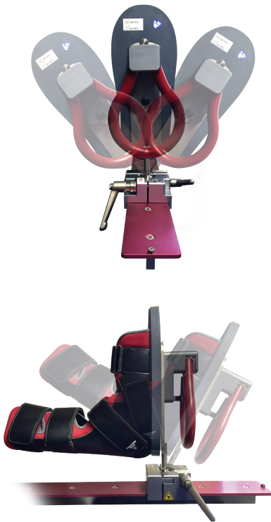
Locking ball and socket joint allows full adjustment of foot plantar flexion, dorsiflexion, inversion and eversion.
